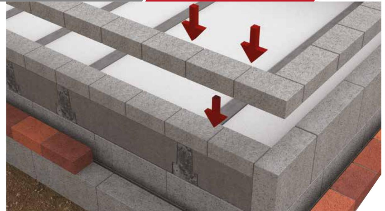
1. Install brick or block courses to bring the perimeter and any internal walls up to finished floor level.
