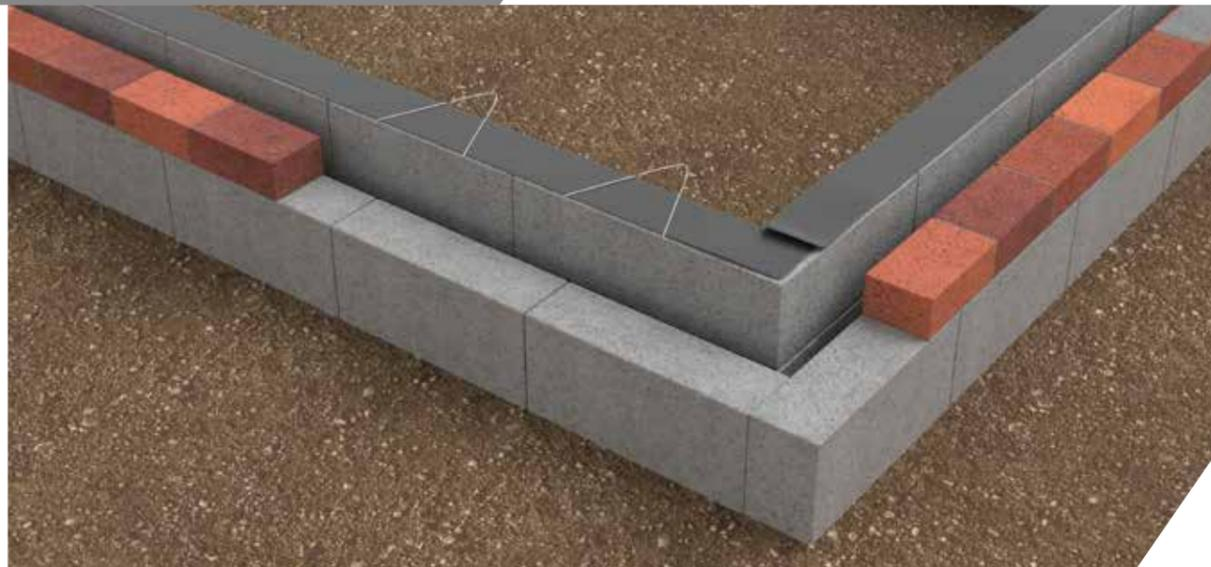
1. Prior to any installation, check that the bearing walls (on which the beams sit) are at the correct height and free of any debris.
